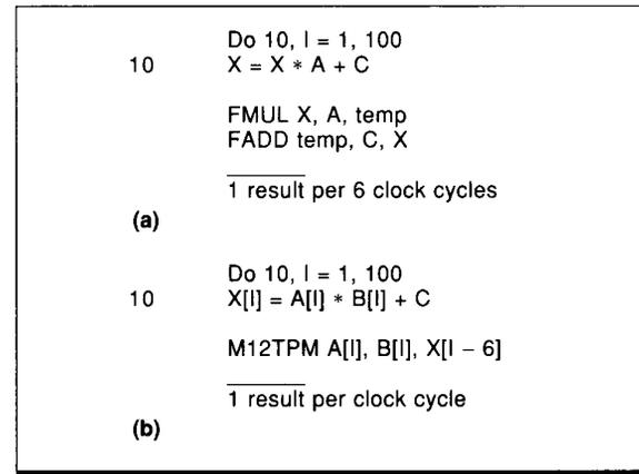
Figure 6. Floating-point execution models: data-dependent code in scalar mode (a) and vector code in pipeline mode (b).
