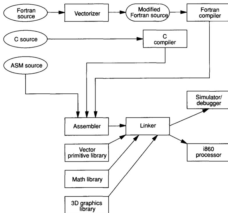
**Figure 12. Software development environment supporting the i860.**
