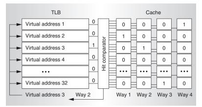
Figure 2. Prevalidated cache tags tied to the TLB determine a hit. The presented virtual address is TLB entry 3. The TLB drives a match line indicating the match to the hit comparator, which reads and compares the way's tags against this match line. The tag in way 2 matches the match line, so way 2 is reported as a hit.
