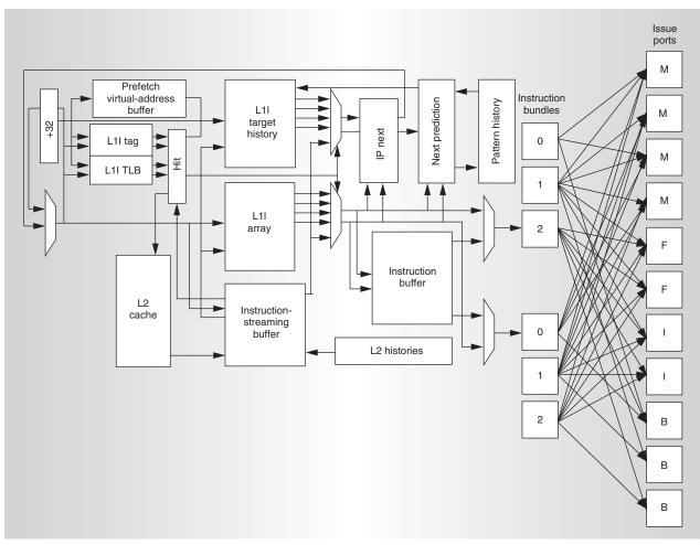
Figure 3. Itanium 2 processor front-end and dispersal-logic design.
