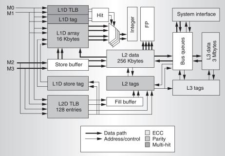
Figure 4. Itanium 2 processor's memory subsystem and system interface.
