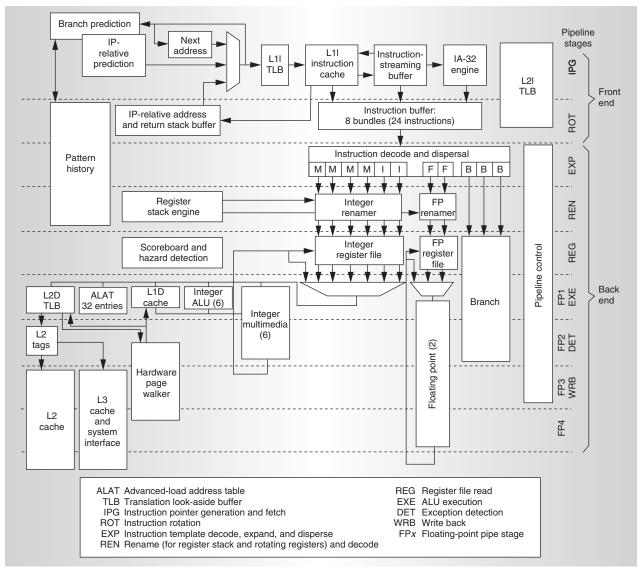
Figure 1. Itanium 2 processor pipeline.
