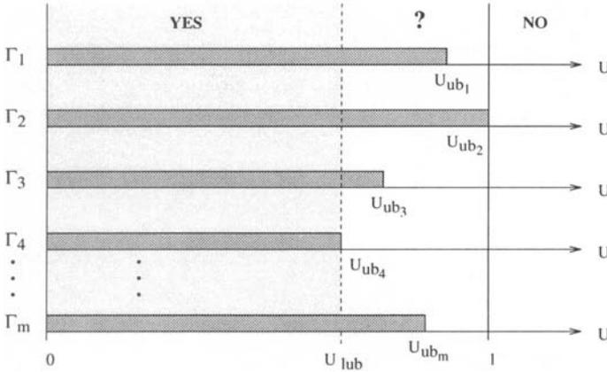
**Figure 4.1** Meaning of the least upper bound of the processor utilization factor.
