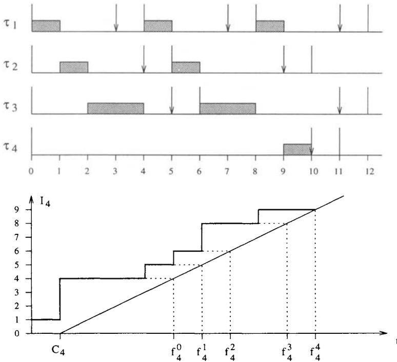
**Figure 4.12** Example of schedule produced by DM.
