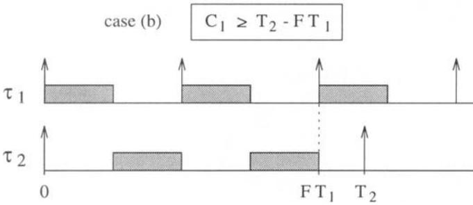
**Figure 4.6** The second request of  $\tau_2$  is released when  $\tau_1$  is active.
