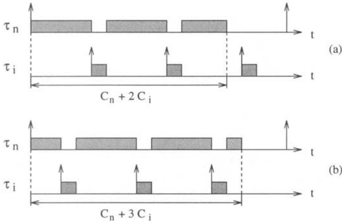
**Figure 4.2** a. The response time of task  $\tau_n$  is delayed by the interference of  $\tau_i$  with higher priority. b. The interference may increase advancing the release time of  $\tau_i$ .
