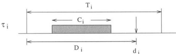
**Figure 4.10** Task parameters in Deadline-Monotonic scheduling.
