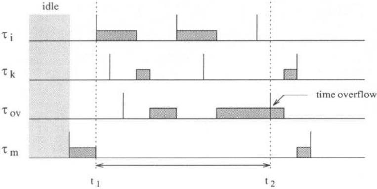
**Figure 4.8** Interval of continuous utilization in an EDF schedule before a time-overflow.
